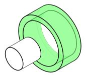
Fig. 1. Three-dimensional sketch of the system composed of a permanent magnet (unshaded, left) and thick coil (shaded, right). The magnet can be modelled as an equivalent cylindrical surface current density, and the coil as a volumetric current density.
