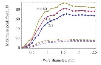
Fig. 11. Maximum peak force  $F_{\rm max}$  versus wire diameter calculated by multiplying the normalised maximum force by the maximum current rating for that wire diameter (Figures 10 and 9, resp.). Solid, labelled lines have a safety factor of 100%; dashed lines represent the same curves using a S=20% safety factor; they exhibit the same shape with a proportionally lower peak amplitude.
