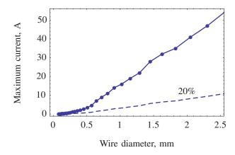
Fig. 10. Typical values for maximum current rating for copper wire of varying diameter [10, adapted], and the same data with a 20% safety factor.
