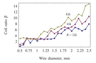
Fig. 12. Optimal values of magnet ratio  $\alpha$  and coil ratio  $\beta$  corresponding to the results shown in Figures 9 and 11 for three resistance values.
