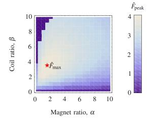
Fig. 8. Peak normalised force  $\hat{F}_{peak}$  as magnet and coil ratios  $\alpha$  and  $\beta$  are varied over a  $20 \times 20$  discrete grid for a specific wire diameter, coil impedance, and magnet volume. Maximum normalised peak force is indicated with a star.
