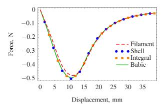
Fig. 5. Comparison between four methods for calculating the force versus axial displacement between a coaxial thick coil and magnet. The discretisation of the filament method incurs a small deviation from the expected results.
