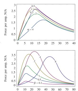
Fig. 7. Normalised force  $\hat{F}_z$  versus displacement calculations for two cases: firstly, varying magnet ratio  $\alpha$  for a fixed coil ratio  $\beta = 1$ , and secondly varying coil ratio  $\beta$  for a fixed magnet ratio  $\alpha = 2$ .
